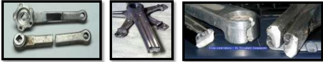
Fig: 1.2 Various Crank Failures
